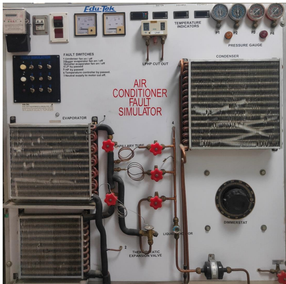
Figure-9.1 Air Conditioner Fault Simulator
