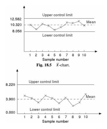
**Comment:** All the points in X-chart are within the control. All the points on the R-chart are also within the control limits. But, there is a dominant up-trend towards right hand side of X-chart. So, we will have to hunt for reasons for variations. This may be due to tool wear, operator fatigue, etc
