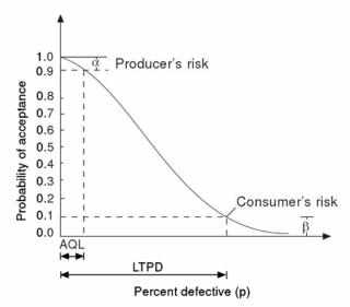
Fig. 18.9 Operating characteristic curve.
