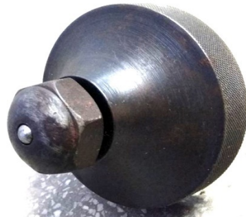
BRINELL HARDNESS TEST ATTACHMENT
