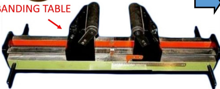
FLEXURAL OR BENDING TEST ATTACHMENT
